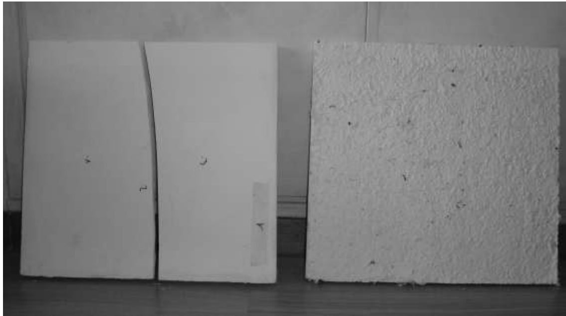
Figure 4 : On the left, gypsum panel at break; on the right, gypsum-LDPE panel at break.
