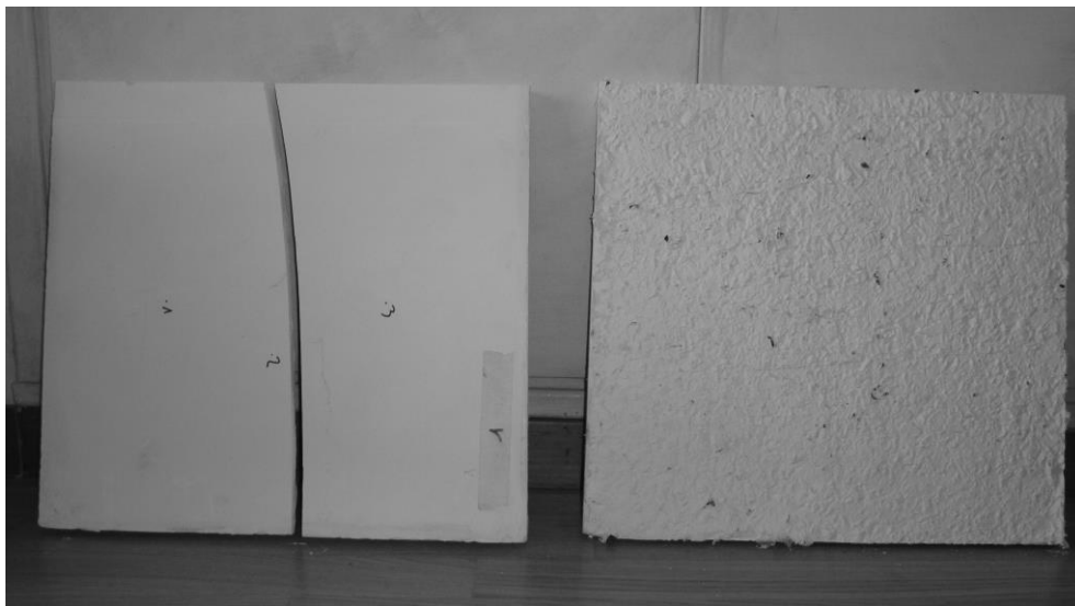
Figure 4. On the left, gypsum panel at break; on the right, gypsum-LDPE panel at break.
