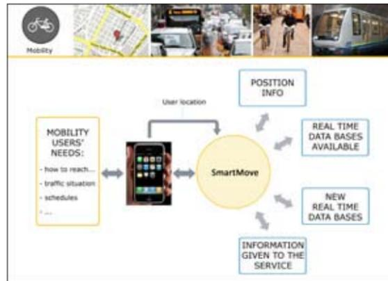
3 Mobility Micro Concept, SmatMove. SmartMove has access to existing databases, to real time sensors in the city and to user generated information. Through these sources it is able to elaborate answers to the users' needs.
